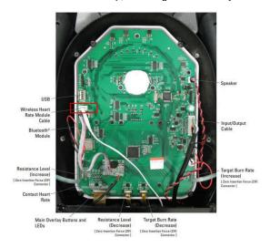
The wireless heart rate module connection is located on the left side of the console board (see red box).
