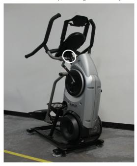
There are two screws located on either side of the console mast. Remove all four screws with the 5mm Allen wrench and carefully remove the console.
