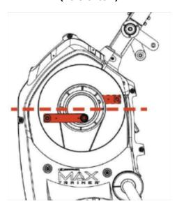
Diagram showing how the crank arms should be oriented when properly installed.
