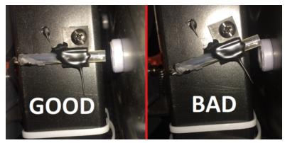
On the left is an example of a properly positioned speed sensor.
