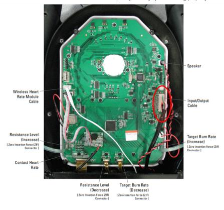
Inspect the input/output wire (circled in red).
