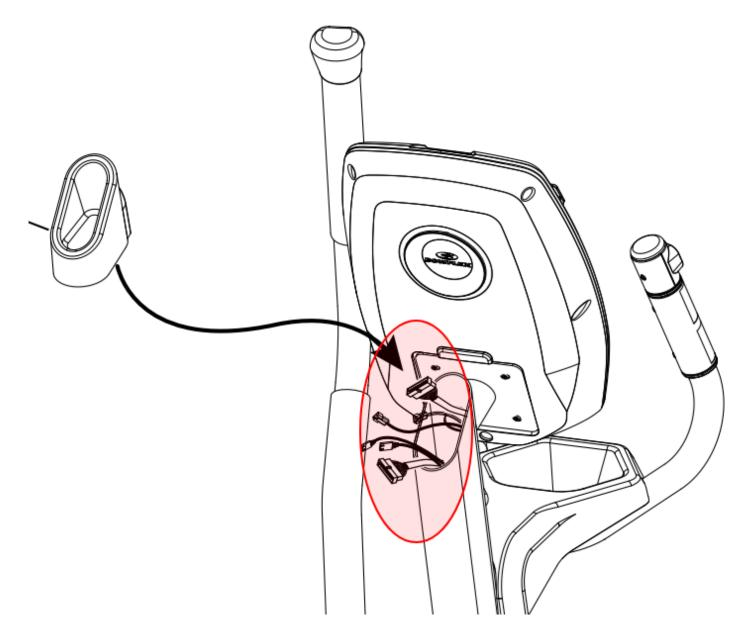
Inspect and reseat the cables located under the console mast end cap.
