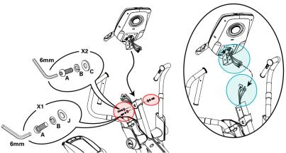
The bolts circled in red need to be removed to access the cables between the console and the console mast.
