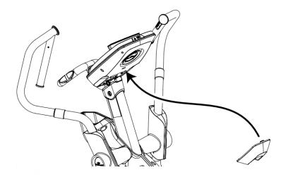
The shroud (pictured in the lower right corner) does not require any tools to remove.
