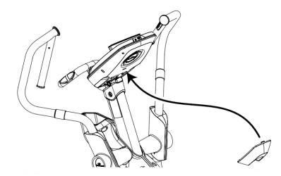
The shroud (pictured in the lower right corner) does not require any tools to remove. Pop it out of place to begin the console removal process.
