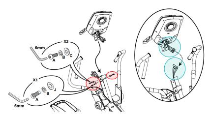
The bolts circled in red need to be removed to access the cables between the console and the console mast. Inspect the cables circled in teal for damage.
