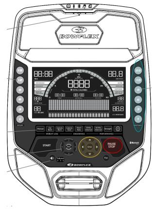
*First, press the button circled in red twice, then attempt to increase the resistance using the buttons circled in teal and gold. Listen for servo motor movement.*
