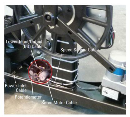
The servo motor is circled in red. Watch the motor for movement as you adjust the resistance.
