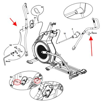
*Remove and disassemble the upper handlebars to inspect the wiring contained inside. The wiring is circled in red and the locations of the bolts are shown using the red arrows.*
