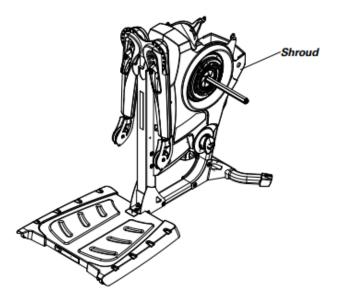
The shroud to remove is labeled in this image. Loosen the screws and reposition, then tighten all hardware.
