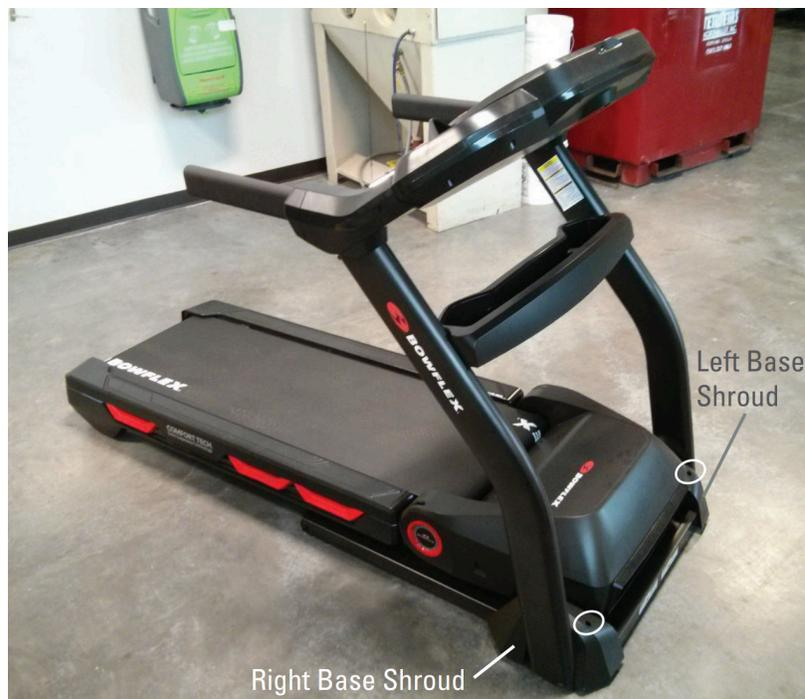
*The base shrouds on either side of the treadmill are attached by the screw circled in white.*
