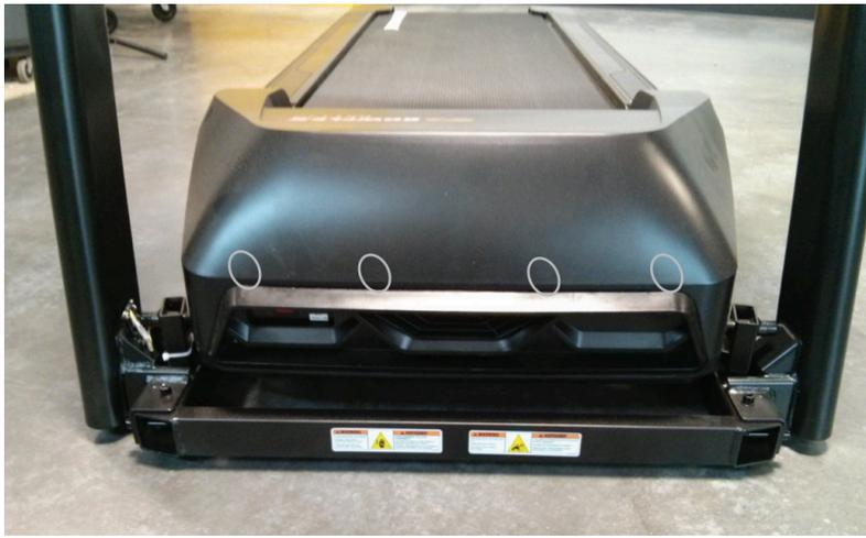
The snaps are located at the front of the treadmill (white ovals) and are not visible from the outside. Be careful to not bend or break the snaps when removing the motor cover.
