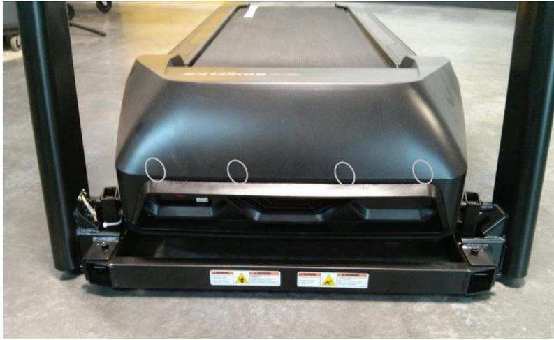
The snaps are located at the front of the treadmill (white ovals) and are not visible from the outside. Be careful to not bend or break the snaps when removing the motor cover.
