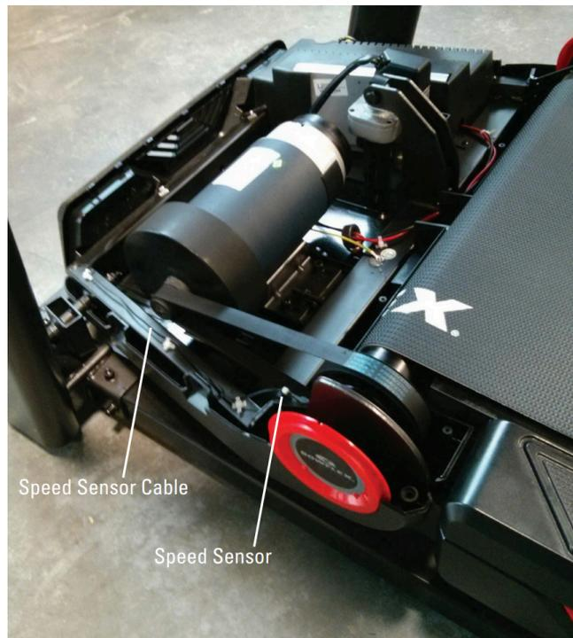
*The speed sensor and cable are located in the motor compartment on the right side.
