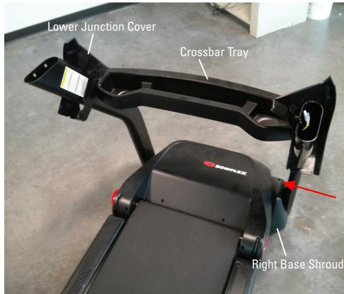
*The base shroud is attached by 1 screw (red arrow).*
