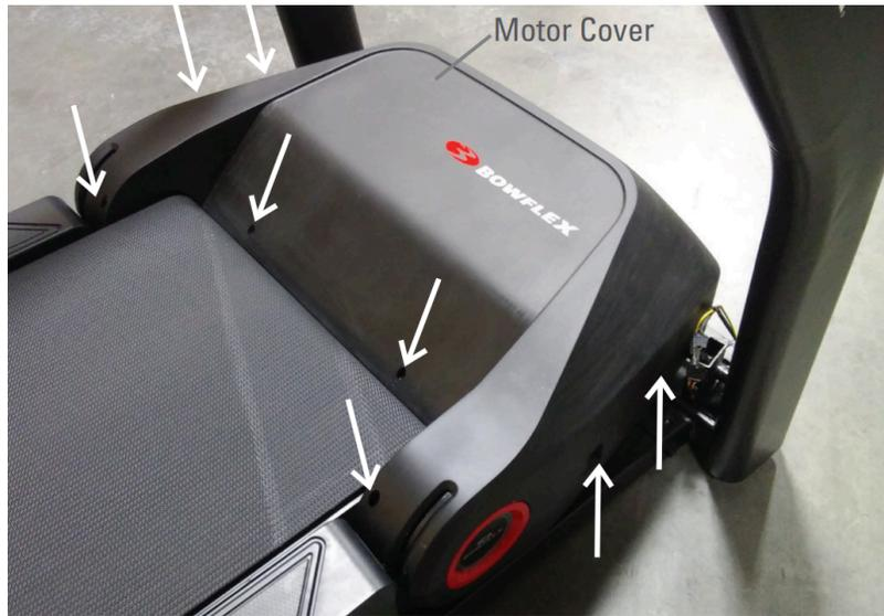
*Remove the 8 screws indicated by white arrows from the top of the motor cover using a Phillips head screwdriver.*
