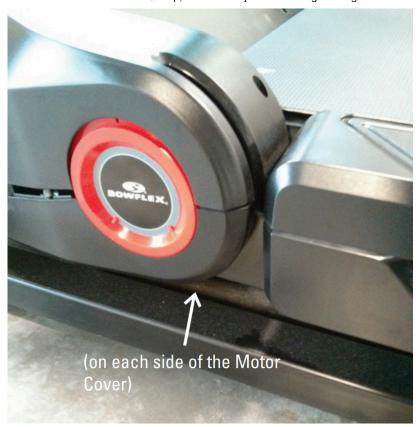
2 screws remain under the motor cover, one on each side. Remove these with a Phillips head screwdriver as well.
