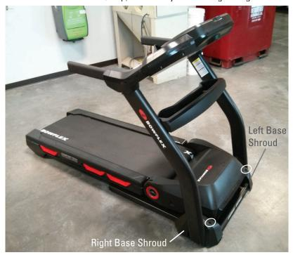
The base shrouds on either side of the treadmill are attached by the screw circled in white. Remove the screw with a Phillips head screwdriver, then remove both base shrouds.
