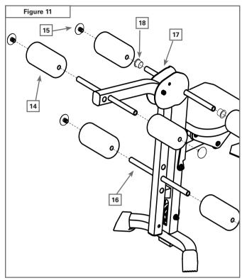
Note: Use a Rubber Mallet to secure the End Caps.
