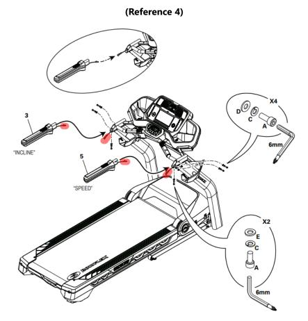
Once the junction covers are removed, the handlebars can be unplugged at the highlighted connections and plugged back in for testing.
