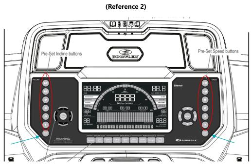
The preset Incline and Speed buttons are circled in red. The CONFIRM INCLINE/SPEED button locations are indicated with the teal arrows.
