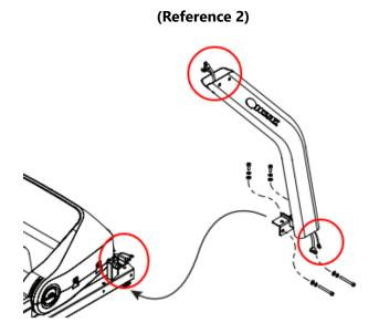
The cable connections to check are circled in red.
