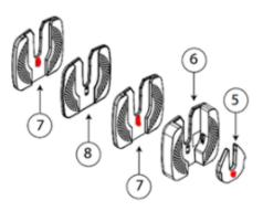
The red markings indicate the position of the selection tabs. The weight plates are installed with the 1.25 lb plate closest to the handle, followed by the 13.75 lb plate, 5 lb plate, 2.5 lb plate, and another 5 lb plate.
