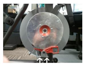
The white arrows indicate the location of the bolts to loosen in order to adjust the brake magnets.
