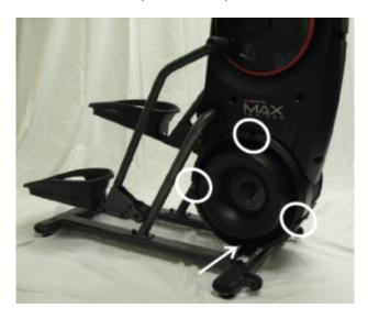
The white circles indicate the location of the 3 upper screws to remove. The white arrow indicates the location of the power inlet wire and bottom screw. Loosen the bottom screw by at least 3 turns, unplug the power inlet wire, then remove the cover.
