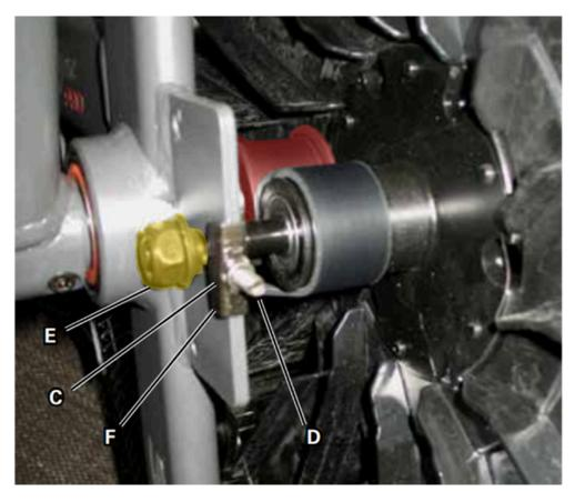
The front idler pulley is highlighted in red and located between the fan and the frame of your bike. The spindle lock nuts to adjust are highlighted in yellow.
